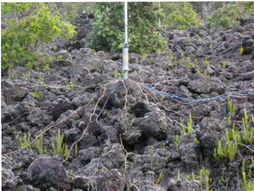
It's hard to get a good earth on a lava flow. 40M phased vertical array at KH7HI
